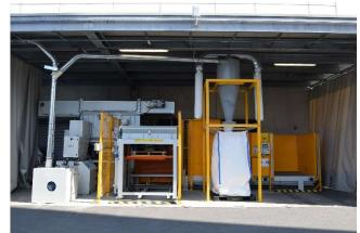
Bag emptying coefficients increase with an emptying mechanism through rotating blades and mixers. Subsequently, a gravimetric fall ensures the separation of most of the material from the bag, released by a counter comb. The pallet loading takes place through a forklift. After the emptying cycle is done, the empty pallet is removed by the forklift. Greater automation can be achieved by integrating an empty pallet stacker and a full pallet accumulator.
